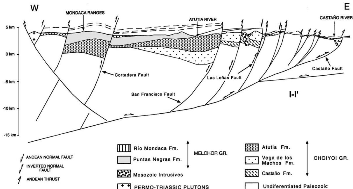
Fig. 3. General geological cross-section of the area. Location in Fig. 1 (Heredia et al., 2002).
